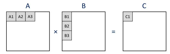
C1 sub-matrix =  $A1 \times B1 + A2 \times B2 + A3 \times B3$  ...
