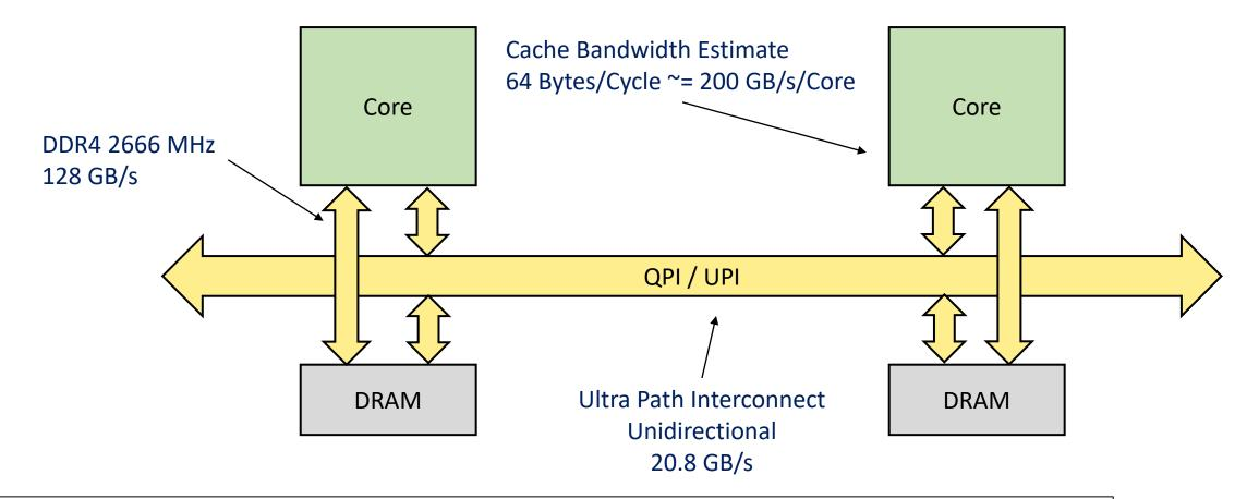
Memory/PCIe controller used to be on a separate "North bridge" chip, now integrated on-die All sorts of things are now on-die! Even network controllers! (Specialization!)
