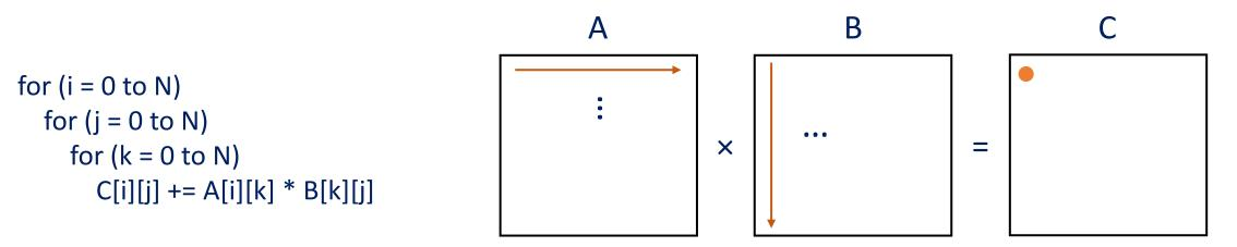
2048\*2048 on a i5-7400 @ 3 GHz using GCC –O3 = 63.19 seconds
